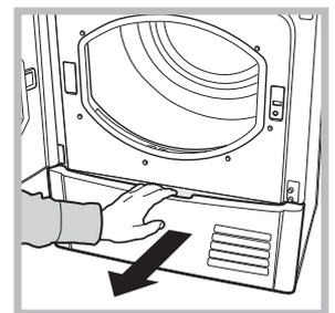
2. Open the condenser cover (see *Picture* below), unlock the three catches by turning them 90° anti-clockwise, then pull on the grip to remove the condenser.
