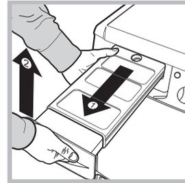
Remove the water container and empty it into a sink or other suitable drain outlet, then replace it correctly. Always check the water container and empty it before starting a new drying cycle.
