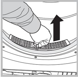
Clean the filter once drying is completed, by rinsing it under running water or cleaning it with a vacuum cleaner. Should the filter become clogged, the flow of air inside the dryer will be seriously hampered: drying times becomes longer and more energy is consumed. Also, the dryer may become damaged.
