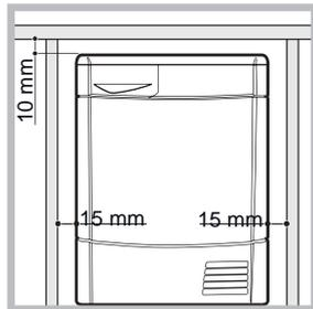
The appliance must be installed with the rear surface placed against a wall.
