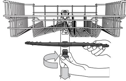
To remove the upper spray arm, turn the plastic locking ring in a clockwise direction. The upper spray arm should be replaced so that the side with the greater number of holes is facing upwards.
