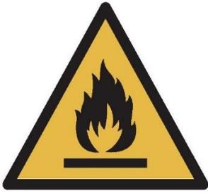
**EN WARNING: Risk of fire/flammable material.** The symbol indicates there is a risk of fire since flammable materials are used. Take care to avoid causing a fire by igniting flammable material.
