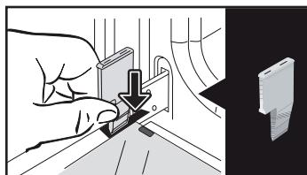
Remove the first clipped glass panel: Using the other wedge (or a screwdriver), press into the slots A to unclip the glass. Remove the glass panel. The door consists of two
