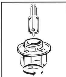
You can replace the bulb yourself. Unscrew the view port and remove the bulb (use a rubber glove, which will make it easier to remove). Insert the new bulb and replace the view port.
