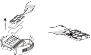
Take out the filters, wipe off the dust with the cleaning brush
