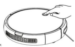
To turn off the robot press the operation button (D) until the operation indicator goes off.
