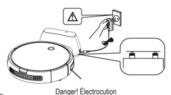
Put the robot in the charging base and ensure that the automatic charging poles are aligned correctly.
