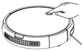
Press the operation button (D) for 2 seconds to awaken the robot. The red indicator will light (Standby mode).
