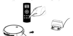
In a low battery condition, the operation button (D) turns blue and blink entering into recharge mode.
