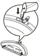
Open the sealed lid of the tank (AG) and introduce water into the tank.
