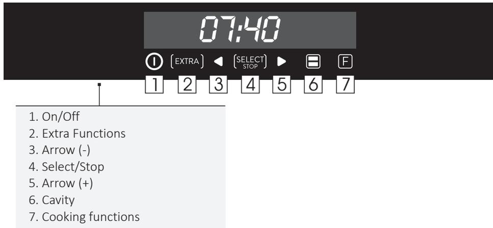
**CAVITY:** When the separator is placed inside the oven, you can select the lower or upper cavity by pressing the
